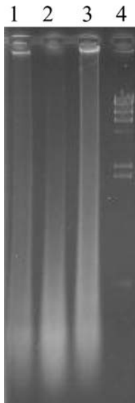
FIG. 1—One and one half percent agarose gel electrophoresis of DNA isolated from a cleaning trial of sheep femur. Lanes 1 – 3 contain 100 ng of DNA (based on OD readings) from bones cooked in water, bleach, and detergent/carbonate respectively. Lane 4 contains a size standard (lambda DNA digested with Hind III), in which the largest band is ~23 kb and the smallest is ~0.56 kb. Note the decreased amount of high molecular weight DNA in the bleach-processed sample, both in the gel and remaining in the well.
